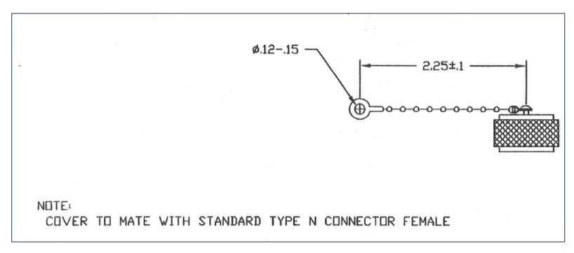
Materials: Nickel-Plated Body, EPDM Gasket, Stainless Steel Bead Chain
