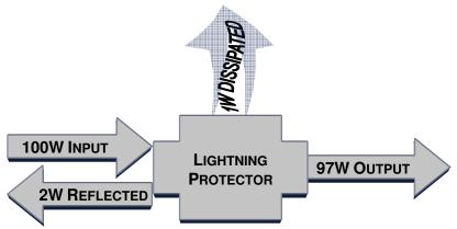
(or return loss). The loss of signal level through the protector is called Insertion
