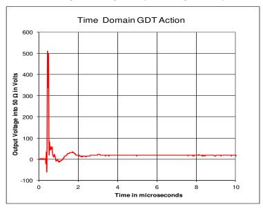
testing. However, since these are suppressors that limit voltage, and are VERY nonlinear, results may not be much different at 3kA versus 20kA.
