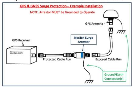
Most GPS Receivers tend to be extremely sensitive to Surge/Overvoltage Energy, and at the same time they are often uptimecritical components. The best way to ensure your equipment is safe and your system is running properly is to use a high quality coaxial surge arrestor, which will protect the receiver from harmful energy.
