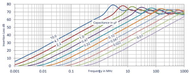
The graph above shows various capacitance values (in  $\mu$ F) and their corresponding Insertion Loss/Filtering Performance For example: a 10 $\mu$ F filter (dark blue, the left-most curve) provides full filtering (60+dB of Loss) by 0.6MHz or 600 $\mu$ KHz
