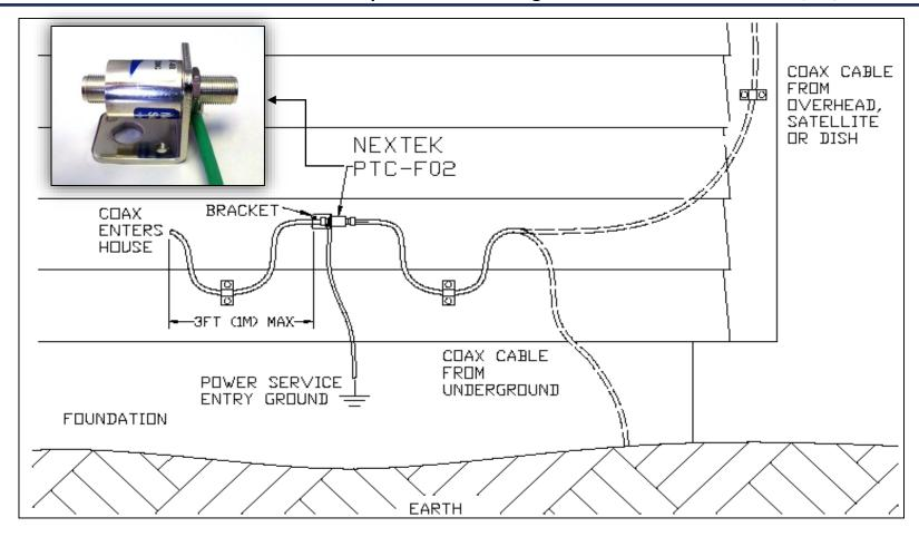
Note: Example shows an Exterior/Outside example, but the PTC-F02 can be installed Inside or Outside.
