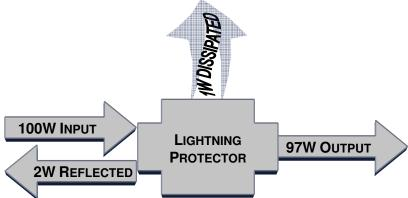
Loss and is measured in decibels (dB). The reflection of a signal back to the source is measured as VSWR (or return loss) also in dB.
