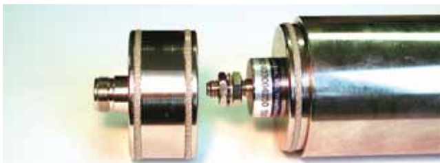
Figure 8. An HPR Filter being installed in test fixture.
